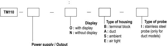
A: Active - 24 Vac/Vdc - 0-10 V P: Passive - 16/30 Vdc - 4-20 mA Example: TM110-POB TH110
